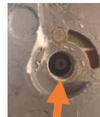
Hole for servo extension. Servo gear shown in the middle.
